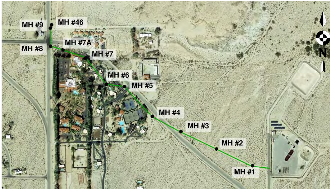
Figure 5-1: Gravity Sewer Main Alignment and Manhole Locations
