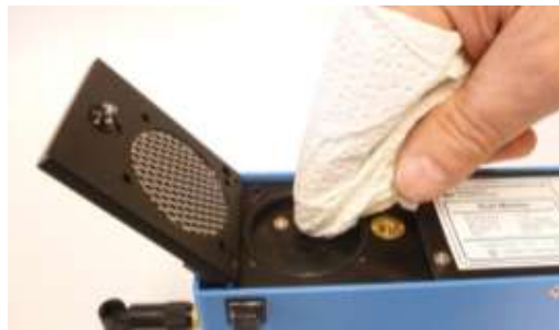
Figure 7-1: Cleaning the filter chamber
