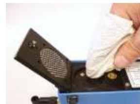
Figure 7-8: Cleaning the filter chamber
