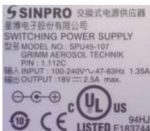
Figure 3-16: Section of the 1112C type plate showing the polarity
