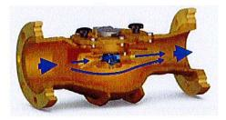
All bearing materials are fortified for minimal wear during high-flow stress. The impeller shaft utilizes tungsten tips to minimize wear and ensure long-term accuracy. The Enduro Model-D meters come with integral flanges (either 6" or 8").
