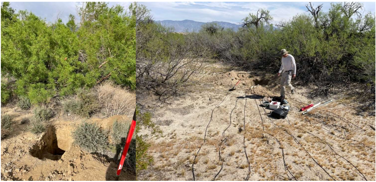
(Left) A soil moisture profile pit at Clark Dry Lake, used to place sensors and establish long-term patterns of soil moisture use by plants. (Right) Soil moisture sensor installation in a profile pit at the Borrego Sink research location.
