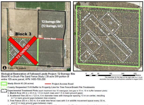
4. Sand Fence (80 m x 123 m; conventional sand fence rows with 12 m bare ground gaps between rows)
