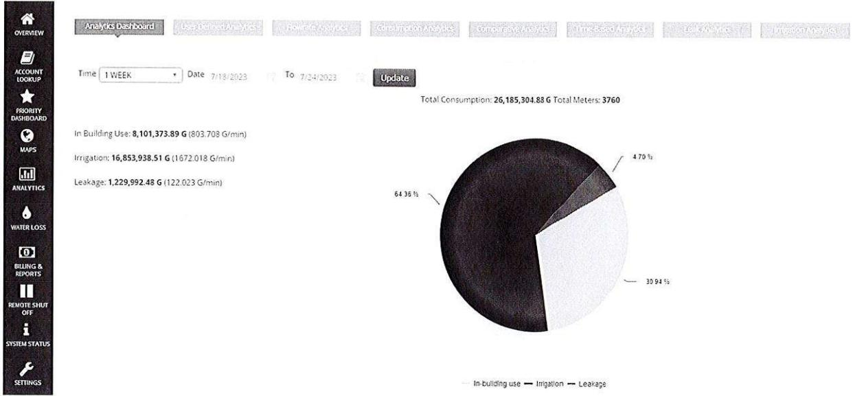
**Flowrate Analytics** – The flowrate analytics page allows the utility to view total consumption by flow rate, either system wide, by a group of meters (i.e., irrigation meters), by meter size, meter type, etc.
